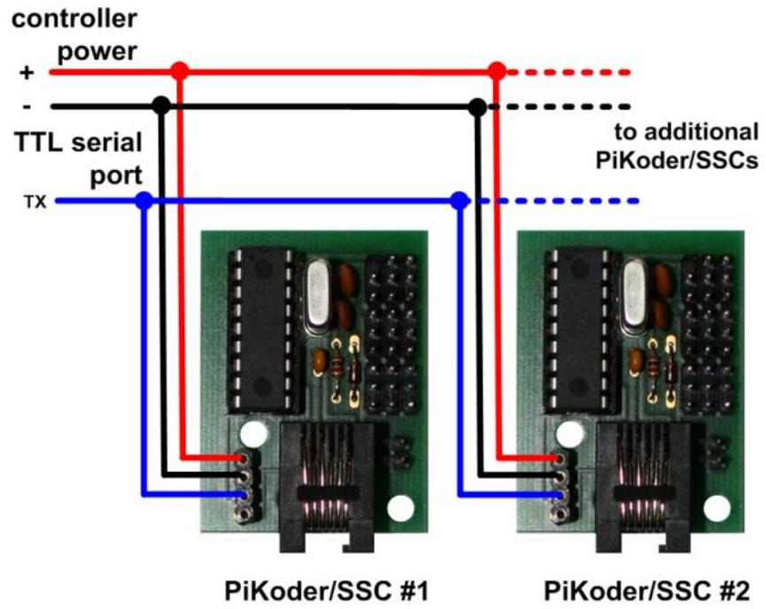
PiKoder/SSC hardware setup for daisy chaining
